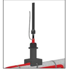
7. Liberally apply RTV over the exposed matrix and leads. Push the rubber boot over the heating cable.
