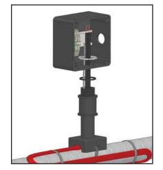
10. Assemble junction box to compression fitting as shown. Tighten locknut until the junction box bottoms out against the lip of the compression fitting.
