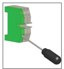
11. Attach 3/4" conduit hub. Use a flathead screwdriver to release the terminal spring clamps and insert cable leads and grounding braid as per wiring diagram on next page. Supply power electrical connections to terminals as shown on wiring diagram on next page. For ATEX and IECEx installations, conduit hub must be an ATEX or IECEx certified component.
