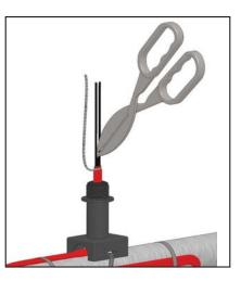
Use tin snips or similar tool to 6. cut excess material from between the buss wires. \*Separate CWM leads
