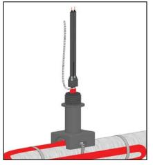
8. Strip each bus wire so that no black matrix material shows above the end of the rubber boot. Trim lead ends as needed.
