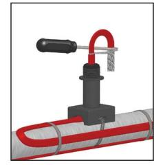
While bending the heating 4. cable, work the cable through the braid opening. Pull the braid tight.
