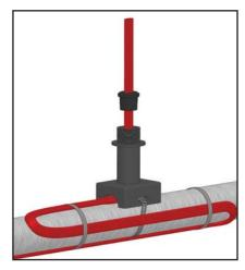
Insert heating cable through 1. pipe standoff and grommet as shown. 8 inches of cable should extend past the grommet. Strap pipe standoff to pipe with pipe strap (Chromalox type PS not included) and attach extra cable to pipe as appropriate. For pipes smaller than 1-1/2" diameter a small pipe adapter (Chromalox model SPA not included) is required.
