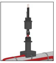
9. Slide compression fittina over cable. Grommet should be placed inside pipe standoff. Termination boot should be spaced 1/2" from sealing grommet.
