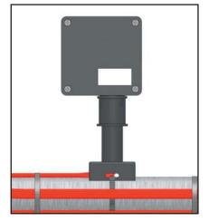
12. Once Locknut is secure and wires are secured in terminal, place cover on box and secure the lid to the box by tightly fastening screws.
