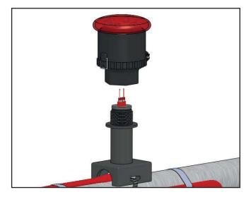
8. Attach LED Assembly to pipe stand off as shown. Liberally apply RTV over the exposed matrix and leads.
