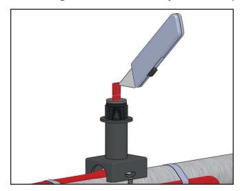
3. 1-1/4 Inches of cable should extend above the grommet. Score the outer insulation 1" from the end of the cable. Lightly cut the outer jacket up the center to end of heating cable and remove the jacket from the cable.
