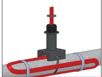
2. Place strain relief part onto cable until it is directly on top of the grommet.
