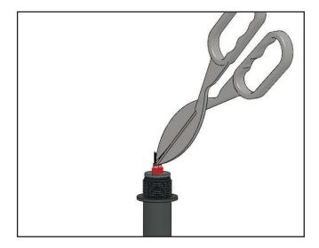
6. Score the inner insulation 1/2" from the end. Lightly cut the inner jacket up the center to end of heating cable and remove the inner jacket from the cable.
