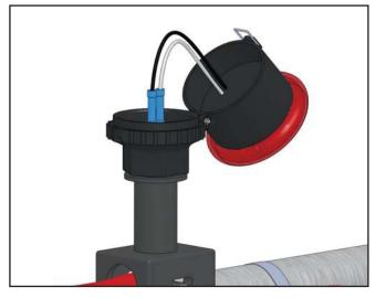
9. Using crimping tool crimp white wire from LED assembly to one buss wire and black wire to the other buss wire.
