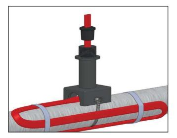
1. Insert heating cable through pipe standoff and grommet as shown. 1-1/2 Inches of cable should extend past the grommet. Strap pipe standoff to pipe with pipe strap (Chromalox type PS not included, UESL to be moiunted vertically only) and attach extra cable to pipe as appropriate. For pipes smaller than 1-1/2" diameter a small pipe adapter (Chromalox model SPA not included) is required.
