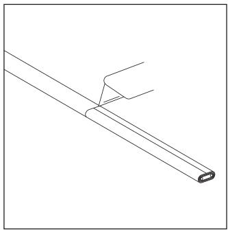
2. Score the outer insulation 7" from the end of the cable. Lightly cut the outer jacket up the center to the end of heating cable and remove the outer jacket from the cable. WARNING: DO NOT CUT METAL BRAID.
