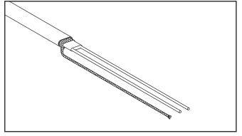
8. Remove the exposed core material and cut 1/4" of the end of each bus wire. \*Skip this step if using CWM-C constant wattage cable.
