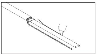
Shave the core material from the outside of each 6. bus wire.
