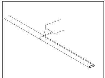
Score the inner insulation 7" from the end. Lightly 4. cut the inner jacket up the center to end of heating cable and remove the inner jacket from the cable.
