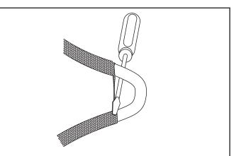
2. While bending the heating cable, work the cable through the braid opening. Pull the braid tight.
