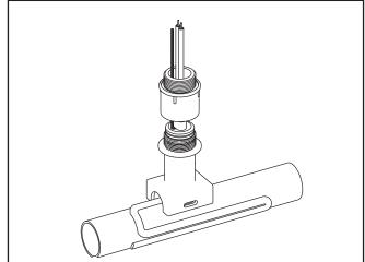
10. Slide compression fitting over cable. Grommet should be placed inside pipe standoff. Termination boot should be spaced 1/2" from sealing grommet. Tighten compression fitting until it bottoms out against pipe standoff.
