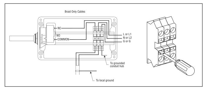
11. Attach 3/4" conduit hub. Use a flat head screwdriver to release the terminal spring clamps and insert cable leads and grounding braid. Please see the electric diagrams below for proper wiring for your application. Attach junction box cover to seal enclosure. Note: The conduit hub should be approved for Class 1, Div. 2; Class II Div. 1 & 2, Class III, Div. 1 & 2, and NEMA 4X rated by a nationally recognized testing laboratory.
