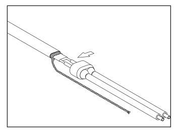
9. Liberally apply RTV over the exposed matrix and leads. Push the rubber boot over the heating cable. Trim lead ends as needed.
