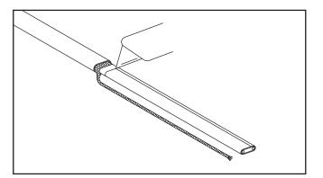
5. Score the inner insulation 6" from the end. Lightly cut the inner jacket up the center to end of heating cable and remove the inner jacket from the cable.
