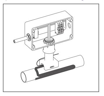
**10.** Assemble junction box to compression fitting as shown. Tighten locknut until the junction box bottoms out against the lip of the compression fitting. To ensure that box is water tight make sure washer for thermostat is against the enclosure.
