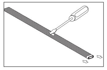
1. For each cable, push braiding back from the end of the cable. 11" from cable end create a bulge. At the bulge, separate the braid to make an opening.
