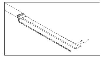
7. Starting at the end of the heating cable, using needle nose pliers or a knife pull each bus wire away from the core material.
