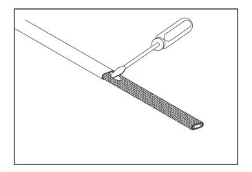
3. Move braid back toward the overjacket, creating a bulge. At the bulge, separate the braid to make an opening.
