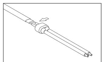
8. Liberally apply RTV over the exposed matrix and leads. Push the rubber boot over the heating cable. Trim lead ends as needed.
