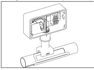
**11.** Assemble junction box to compression fitting as shown. Tighten locknut until the junction box bottoms out against the lip of the compression fitting. To ensure that box is water tight make sure washer for thermostat is against the enclosure.
