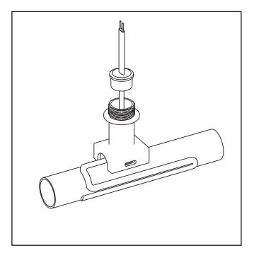
1. Insert heating cable and grommet as shown. 8" of cable should extend past the grommet. Attach the pipe standoff to the pipe with a pipe strap (Chromalox type PS not included) as shown. Attach extra cable to pipe as appropriate. For pipes smaller than 1-1/2" diameter optional small pipe adapter (Chromalox model SPA not included) is required.
