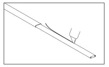
5. Shave the core material from the outside of each bus wire.
