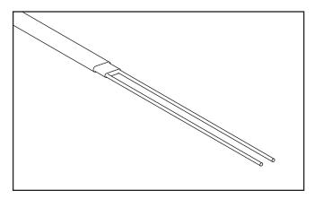
7. Remove the exposed core material and cut 1/4" off the end of each bus wire. \*Skip this step if using CWM-C constant wattage cable.
