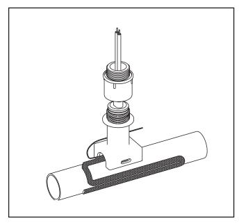
9. Slide compression fitting over cable. Grommet should be placed inside pipe standoff. Termination boot should be spaced 1/2" from sealing grommet. Tighten compression fitting until it bottoms out against pipe standoff.
