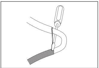
4. While bending the heating cable, work the cable through the braid opening. Pull the braid tight.
