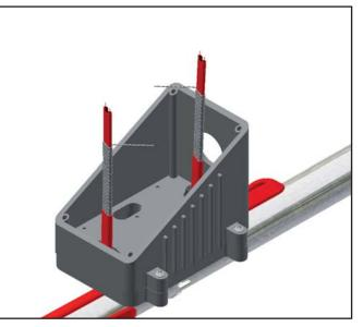
8. Insert the bared ends of the conductors and the braid into the openings in the terminal block. Tighten screws firmly to hold the wires and braid in place.
