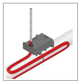
4. Score the outer insulation 7 inches from the end of the cable. Remove the jacket to expose the metal braid. CAUTION: When removing outer jacket, be careful not to damage the braid of the base cable insulation. NOTE: If using braid only cable (-C) skip this step.
