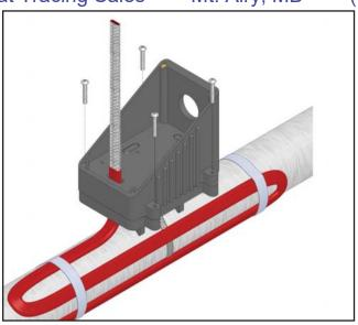
Feed cables through the corresponding holes in the box and secure box to base using all four screws.
