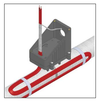
7. Using standard electrical cutters, cut a 3/4 in long notch out of the cable between the conductor wires. Bare a 3/8 inch length of each conductor by stripping off the outside insulation and the inner black core material.
