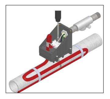
11. Mount terminal block to bottom of the box by driving the self-tapping screw (Item 5) provided into the mounting hole as shown.
