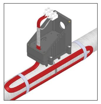
8. Insert the bared ends of the conductors and the braid into the openings in the terminal block. Tighten screws firmly to hold the wires and braid in place.
