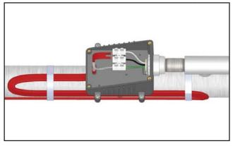
10. Strip 3/8 inch length of each power wire and connect to unused side of terminal block as shown. Tighten screws firmly to hold wires in place.
