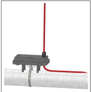
3. Slide cable grommet over the end of the cable and insert it into the opening in the base. Secure the base to the pipe by threading the appropriate sized pipe strap through the slot in the mounting plate. Tighten the pipe strap until the base is securely attached to the pipe.
