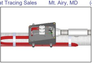
9. Connect conduit hub (Chromalox CCH, CH -75 or equal) to the box. Attach conduit to hub and bring power leads into box.
