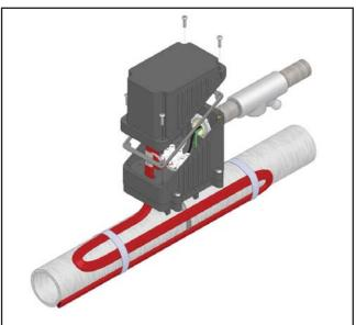
12. Carefully push the all wires into the box and secure the lid to the box. Make sure water tight rubber gasket (Item 8) is in place.
