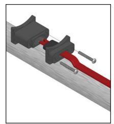
Slide the end cap over the grommet. Using a screwdriver, connect the pressure plate to the end cap.
