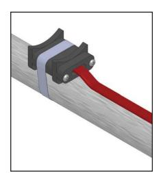
Using a fastening device, fiber reinforced electrical tape (Chromalox FT-3 or equal), secure the assembly to the pipe. Wrap the tape around the assembly between the legs.
