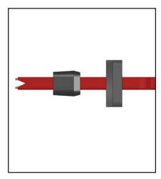
Using standard electrical cutters, cut a "VEE" notch between the buss wires.
