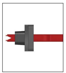
Slide the pressure plate and grommet towards the end of the cable leaving 5/8" of the cable past the end of the grommet.
