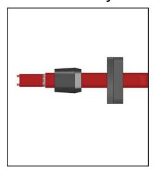
Score the outer jacket one inch from the end of the cable. Remove the jacket to expose the braid. Unravel and trim the braid flush with the outer jacket. Pull any strands of braid back towards the outer jacket.
