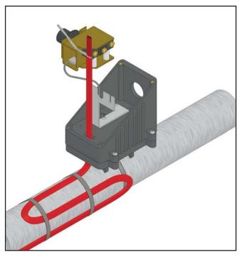
Insert the bared ends of the conductors and the braid into the openings in the terminal block. Tighten screws firmly to hold the wires in place. Attach UL certified conduit to hub and bring power leads into box. Strip 3/8" length of each power wiring. Connect conduit hub (Chromalox CCH-1, CH-75 or equal) to the box. Attach conduit to hub and bring 8" of power leads into the box.
