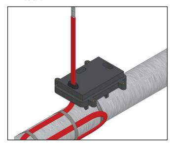
5. Feed the capillary of the thermostat through the side hole of the box. Slip the grommet over the capillary between the box and the base. Feed the cable through the end hole in the box. Allow 3/4" of stainless steel capillary to extend above the bottom of the box. Secure box to base using all four larger (8-32) screws.
