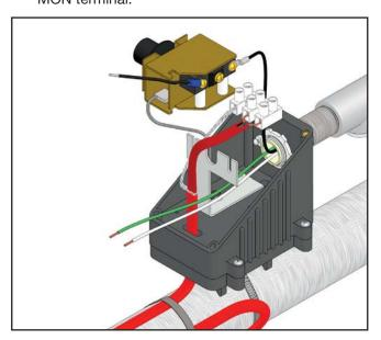
10. Insert the bared end of the grounding wire into the opening of the terminal block which is opposite of the braid. Insert the ends of the other hot (or neutral) wire and the eight inch long wire into the two (2) remaining openings in the terminal block. Tighten screws firmly to hold conductors in place.
