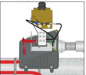
11. Mount terminal block to bottom of the box by driving the self-tapping screw provided into the mounting hole as shown. Thread the screws into the outside pair of mounting holes of the thermostat leaving approximately 1/8" of thread. Slide the screws into the slots in the mounting bracket. Push the thermostat down as far as it will go and tighten the screws firmly.
