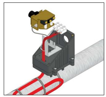
9. Remove the screw and collar from the NORMAL-LY CLOSED terminal of the thermostat. Discard the collar. Push the screw through the opening in the connector attached to the insulated wire and screw it back into the NORMALLY CLOSED terminal. Crimp the ring connector onto the end of the "HOT" conductor. Remove the screw and collar from the COMMON terminal. Discard the collar and push the screw through the opening in the ring connector. Drive the screw back into the COM-MON terminal.
