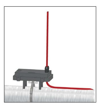
3. Slide cable grommet over the end of the cable and insert it into the opening in the base. Secure the base to the pipe by threading the appropriate sized pipe strap through the slot in the mounting plate. Tighten the pipe strap until the base is securely attached to the pipe.
