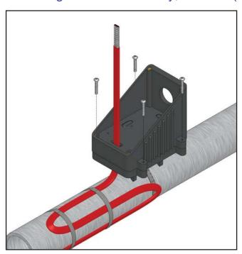
Feed cables through the corresponding holes in the box and secure box to base using all four of the 1" long screws.
