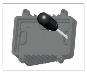
1. Use a hammer and screwdriver to punch out the knockouts on the bottom of the box which correspond to the openings in the base through which the heating cable passes. Only punch out the knockouts that are to be used. If one is mistakenly punched, blank grommets can be ordered to reestablish the water tight seal.
