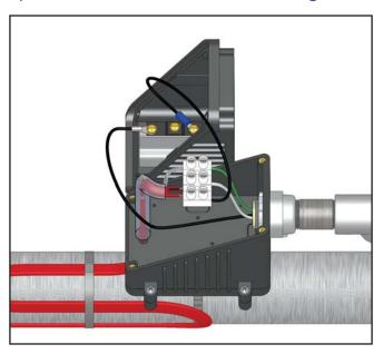
10. Insert the bared end of the grounding wire into the opening of the terminal block which is opposite of the braid. Insert the ends of the other hot (or neutral) wire and the eight inch long wire into the two (2) remaining openings in the terminal block. Tighten screws firmly to hold conductors in place. See wiring diagram on page 7.
