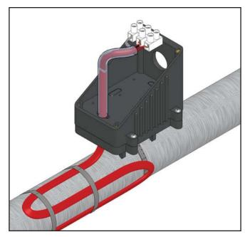
Slide the 6" insulation tubing over the cable. Insert the bared ends of the conductors and the braid into the openings in the terminal block. Tighten screws firmly to hold the wires in place. Connect conduit hub (Chromalox CCH, CH-75 or equal) to the box. Attach conduit to hub and bring power leads into box. Strip 3/8" length of each power wiring. Crimp the ring connector onto the end of the "Hot" conductor.
