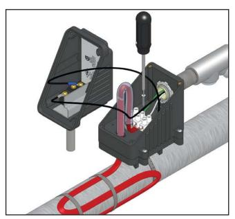
11. Mount terminal block to bottom of the box by driving the self-tapping screw (Item 11) provided into the mounting hole as shown.
