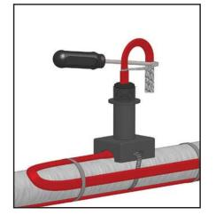
4. While bending the heating cable, work the cable through the braid opening. Pull the braid tight.
