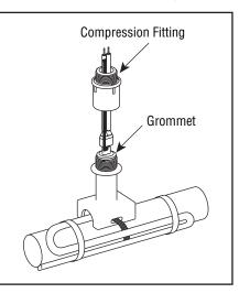
9. Slide compression fitting over cable. Grommet should be placed inside pipe standoff. Termination boot should be spaced 1/2" from sealing grommet. Tighten compression fitting until it bottoms out against pipe standoff.
