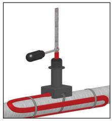
3. Move braid back toward the overjacket, creating a bulge. At the bulge, separate the braid to make an opening.
