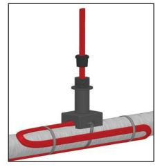
1. Insert heating cable through pipe standoff and proper grommet as shown. 8 inches of cable should extend past the grommet. Strap pipe standoff to pipe with pipe strap (Chromalox type PS not included) and attach extra cable to pipe as appropriate. If the provided RTD is to be fed through the standoff pipe, a small slice will need to be made to the outer edge of the top of the grommet. For pipes smaller than 1-1/2" diameter a small pipe adapter (Chromalox model SPA not included) is required.
