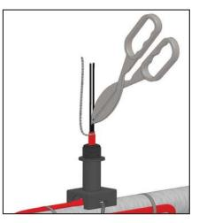
6. Use tin snips or similar tool to cut excess material from between the buss wires.
