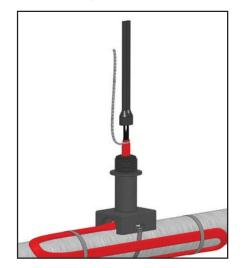
7. Liberally apply RTV over the exposed matrix and leads. Push the rubber boot over the heating cable.
