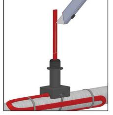
2. Score the outer insulation 7 inches from the end of the cable. Lightly cut the outer jacket up the center to the end of heating cable and remove the outer jacket from the cable. WARNING: DO NOT CUT METAL BRAID.
