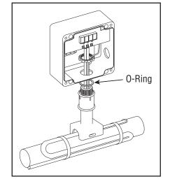
10.Seat O-Ring into compression fitting groove at base of threads. Ensure O-Ring is not twisted. Assemble junction box to compression fitting as shown. Tighten locknut until the junction box bottoms out against the lip of the compression fitting.
