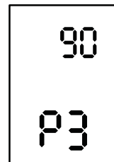
Time delay to stop heaters
