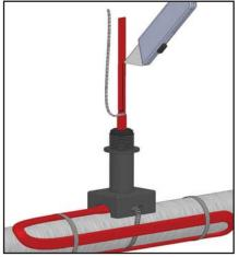
5. Score the inner insulation 6 inches from the end. Lightly cut the inner jacket up the center to end of heating cable and remove the inner jacket from the cable.
